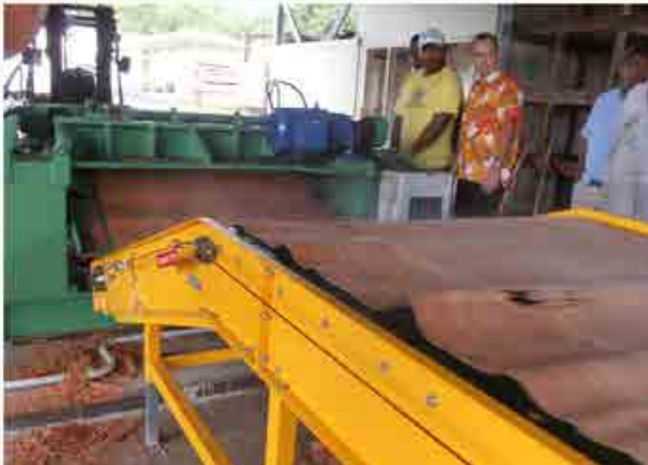
Cocowood Veneer peeled during the trial run of the lathe.
