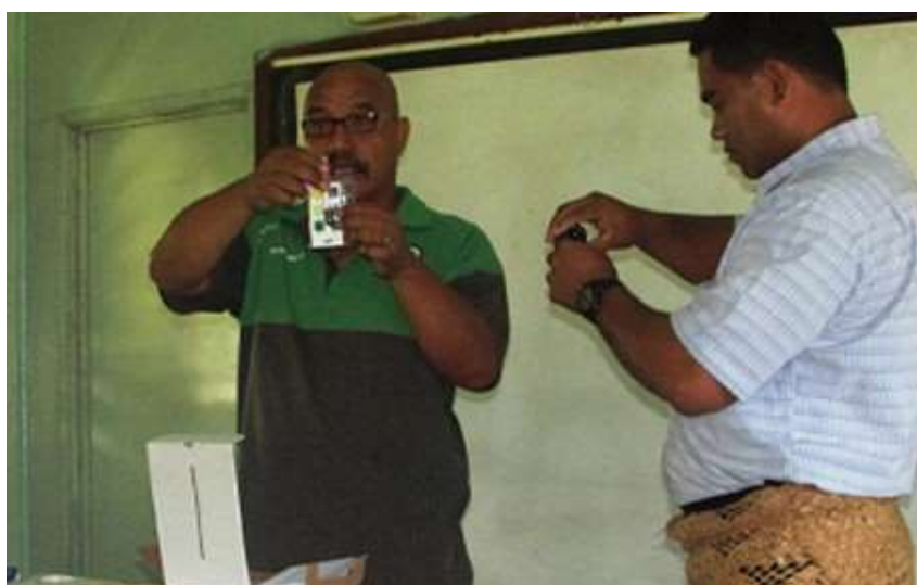
Figure 6. Soil test kits involve mixing the soil with particular solutions and comparing the colour of the mixture with a standard chart. Different solutions are used to test pH and each of the elements.
